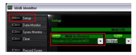
By default, the **MIDI In Device** should be **Open**. This is necessary for the software to be able to read the incoming data from the DJ Console.
