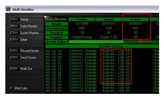
This test can also help determine if some of the controls of the DJ Console are not working correctly. For example, if the crossfader is only halfway to his course but already displays its maximum value of 127.
