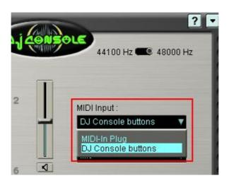
**NOTE:** You could also test an external controller (such as a keyboard) connected to the MIDI IN of the DJ Console. In this case, select **MIDI-In Plug.**
