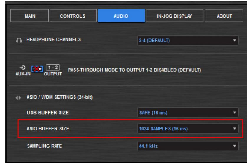
As the name implies, this setting modify the length of the buffer between the audio application and the driver. This basically indicates how much audio and MIDI data can temporarily be stored while the computer is handling other tasks (displaying graphics on screen, reading and writing to the hard drive, etc).
