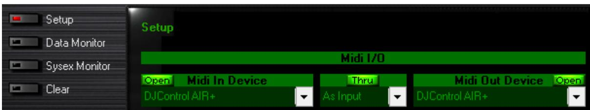
By default, the **MIDI In Device** should be **Open**. This is necessary for the software to be able to read the incoming data from the controller.
