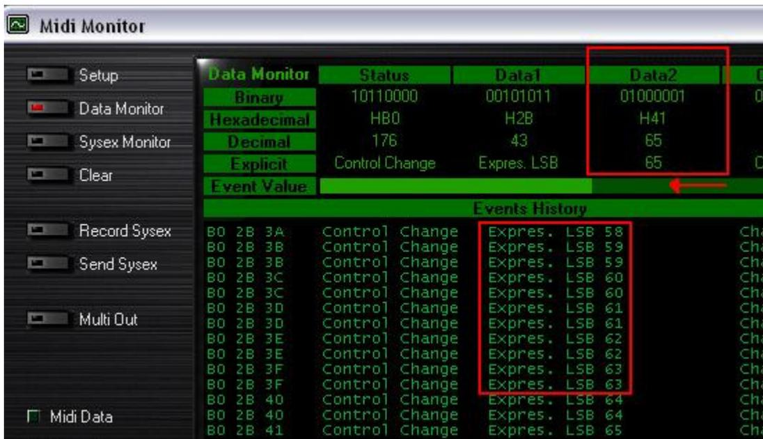
This test can also help determine if some of the controls of the DJ Console are not working correctly. For example, if the crossfader is only halfway to his course but already displays its maximum value of 127.
