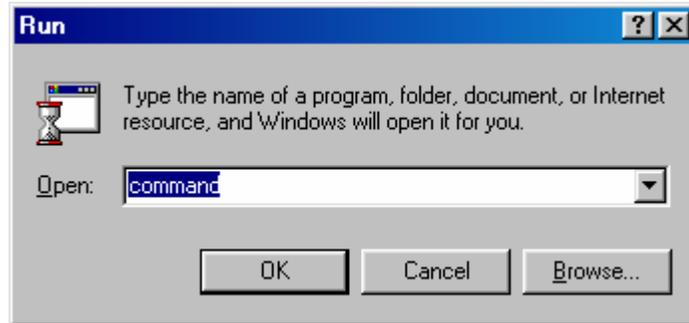
In the window that is displayed, enter the command "ipconfig" and then press the "Enter" key.
