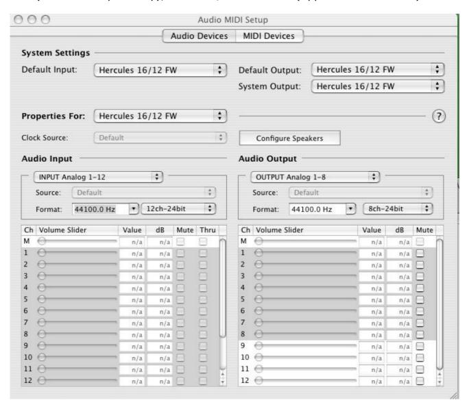
When powered ON, the 16/12 FW should be seen as the default audio INPUT and OUTPUT, but if not, you can use the drop menu to select it.
