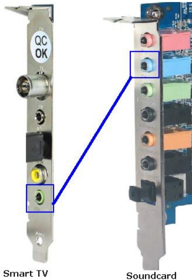
**2** - - You have configured your soundcard so that the LINE IN is selected as Recording source input, and that it is not muted on playback
