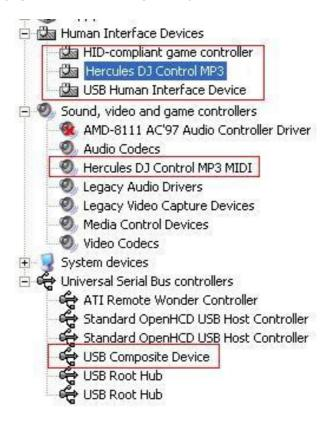
If **Hercules DJ Control MP3** (here in blue) is recognized as another **USB Human Interface Device**, you will not be able to use the DJ Control as a MIDI controller. You will need to reinstall the driver
