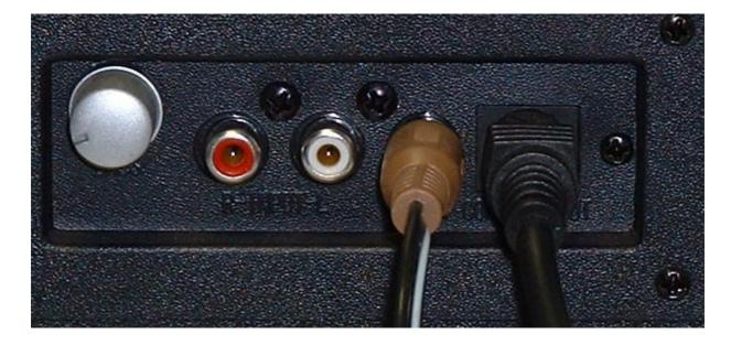
Next, connect the input cable to the RED and WHITE input socket:
