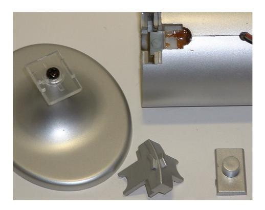
All that is left to do is to re-assemble everything. Start by inserting the  $\mathbf{``O''}$  where the base use to be, at the bottom of the speaker:
