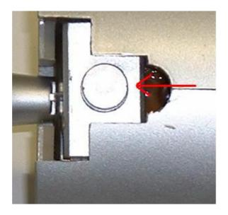
Next, remove de second piece, "O", by sliding it backward, and remove the base, sliding upward. You will then obtain de following pieces:
