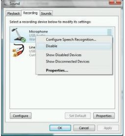
3. The Line input is enabled as soon as the microphone input is disabled.
