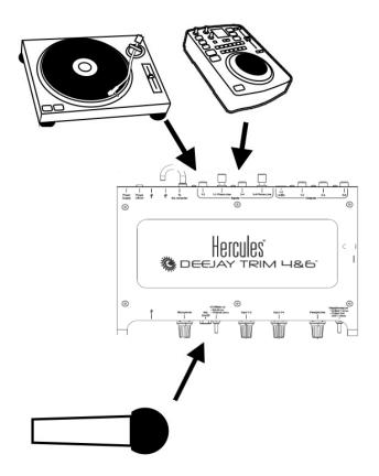
Many types of audio sources devices can be connected to your DeeJay Trim. Whether you want to use the songs from your MP3 player or a Timecoded CD, it is important to define your audio source type (i.e. the correct output level for the device you are connecting) **before** making the connection to the DeeJay Trim. Doing so will avoid possible audio issues such as distorted sound and preserve your ears.
