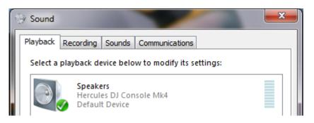
When connected, the DJ Console should be seen as the default **Sound Playback** and **Sound Recording**. If you wish to use any other soundcard for applications other than DJ (Chat, movies, etc), you can select it from this menu.
