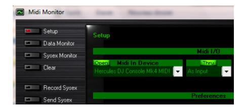
By default, the **MIDI In Device** should be **Open**. This is necessary for the software to be able to read the incoming data from the DJ Console.
