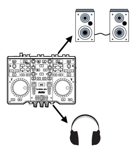
You can use either the mini-jack or RCA connectors of **Output 1-2** to connect regular computer speakers or a home sound system on the back of the Mk4
