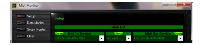
By default, the **MIDI In Device** should be **Open**. This is necessary for the software to be able to read the incoming data from the DJ Console.
