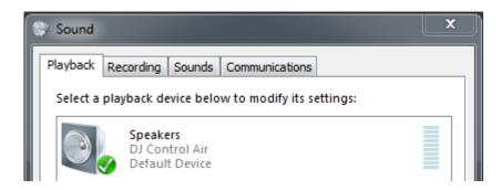
When connected, the DJ Console should be seen as the default **Sound Playback**. If not, you can use the drop menu to select it. You will notice that it does not appear under **Recording** since the device does not have any audio input.
