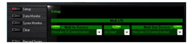
By default, the **MIDI In Device** should be **Open**. This is necessary for the software to be able to read the incoming data from the controller.
