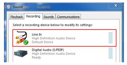
**Line In** should appear available as recording source for the computer's soundcard (the name may vary depending on models and manufacturers).
