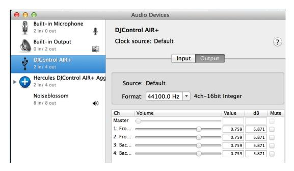
Both Hercules DJControl AIR+ and Hercules DJControl AIR+ Aggregate Device should be present. This is normal and necessary for some DJ software to use all the outputs of the DJControl AIR+.
