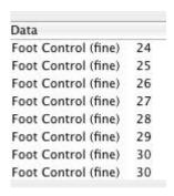
This test can also help determine if some of the controls of the DJ Control are not working correctly. For example, if the Crossfader is only halfway to his course but already displays its maximum value of 127.
